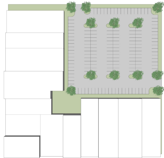
Figure 3.16 | Surface Parking Configuration Behind Buildings
